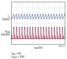
Switching Waveforms (in Deep Burst Mode)
