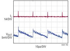
Figure 2. Burst Mode Operation
