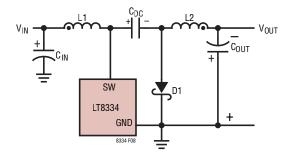
Figure 8. A Simplified Inverting Converter
