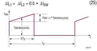
Figure 7. The Switch Current Waveform of the SEPIC Converter
