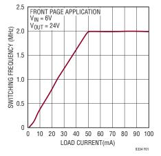
Figure 1. Burst Frequency vs Load Current
