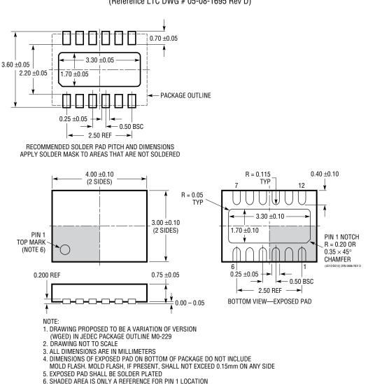
DE/UE Package 12-Lead Plastic DFN (4mm × 3mm) (Reference LTC DWG # 05-08-1695 Rev D)
