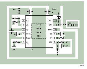
Figure 5. Suggested Boost Converter Layout
