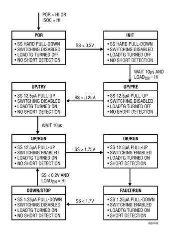
Figure 8. Start-Up and Fault Sequence
