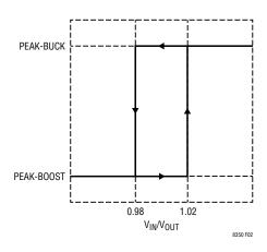
Figure 2. Current Mode vs V<sub>IN</sub>/V<sub>OUT</sub> Ratio
