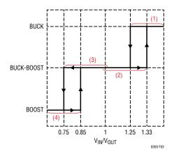
Figure 3. Operation Region vs V<sub>IN</sub>/V<sub>OUT</sub> Ratio
