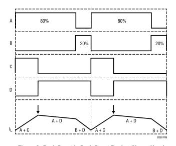
Figure 6. Peak-Boost in Buck-Boost Region (V<sub>IN</sub> <~ V<sub>OUT</sub>)
