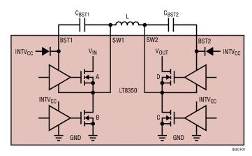
Figure 1. Power Stage Schematic
