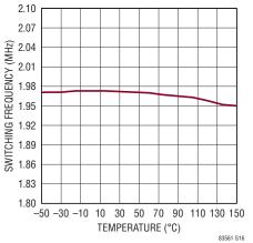
Switching Frequency (400kHz) vs Temperature
