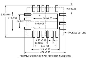
APPLY SOLDER MASK TO AREAS THAT ARE NOT SOLDERED
