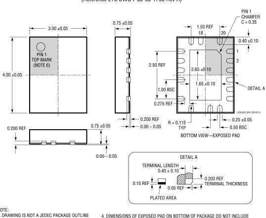
**UDCM Package** 20-Lead Plastic Side Solderable QFN (3mm × 4mm) (Reference LTC DWG # 05-08-1793 Rev A)
