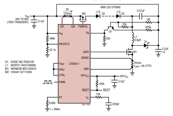
48W, 2MHz Buck-Mode LED Driver with High Dynamic Range PWM Dimming
