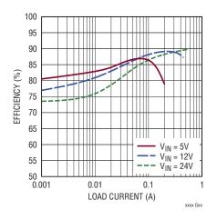
Figure 3. Efficiency vs Load Current
