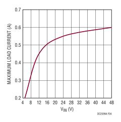
Figure 4. Maximum Load Current vs Input Voltage
