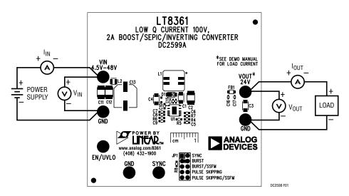
Figure 1. DC2599A Proper Equipment Setup
