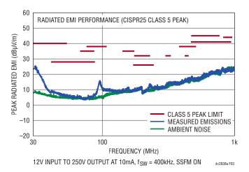
Figure 3. CISPR25 Radiated Emissions Test, Peak Detection
