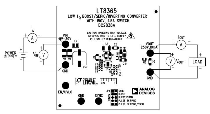
Figure 1. Proper Equipment Setup
