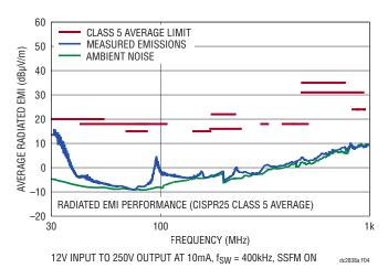
Figure 4. CISPR25 Radiated Emissions Test, Average Detection
