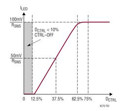
Figure 2. Duty Ratio CTRL Range
