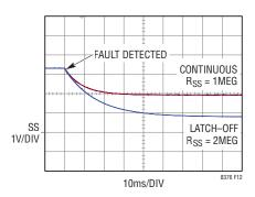
Figure 12. Latch-Off Response to a Fault
