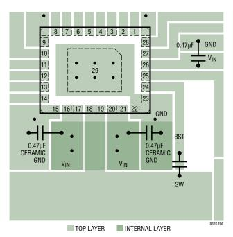
Figure 6. Placement of Input Capacitors
