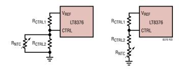
Figure 3. Setting CTRL with NTC Resistors
