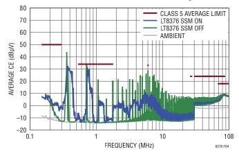
Figure 4. Typical Average Conducted Emissions
