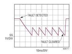
Figure 11. Hiccup Response to Fault
