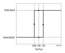
Figure 2. Current Mode vs V<sub>IN</sub>/V<sub>OUT</sub> Ratio
