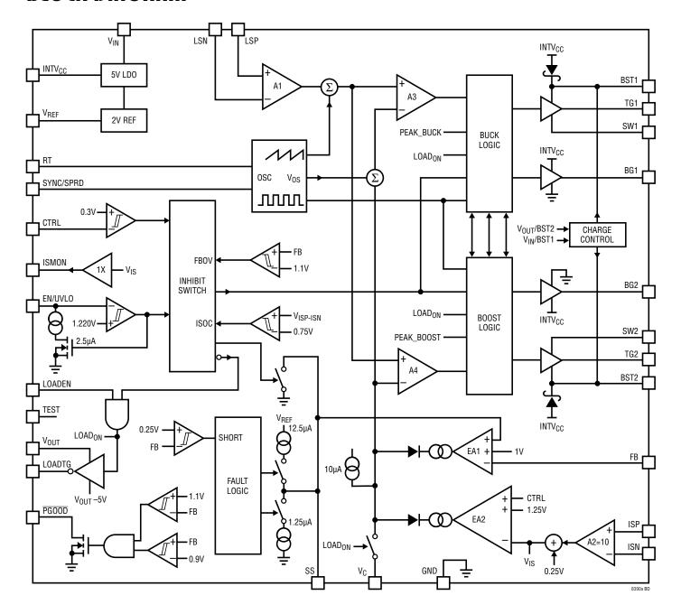
The LT8390A is a current mode DC/DC controller that can regulate output voltage, input or output current from input voltage above, below, or equal to the output voltage. The ADI proprietary peak-buck peak-boost current mode control scheme uses a single inductor current sense resistor and provides smooth transition between buck region, buck-boost region, and boost region. Its operation is best understood by referring to the Block Diagram.
