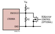
Figure 12. V<sub>IN</sub> Undervoltage Lockout (UVLO)
