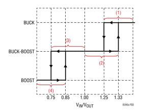
Figure 3. Operation Region vs V<sub>IN</sub>/V<sub>OUT</sub> Ratio
