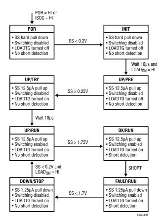
Figure 8. Start-Up and Fault Sequence
