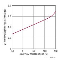
Figure 11. Normalized  $R_{DS(ON)}$  vs Temperature
