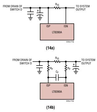
Figure 14. Programming Output Current Limit
