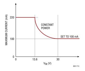
Figure 13. REG LDO Current Limit vs  $V_{BIAS}$  Voltage
