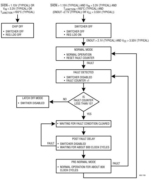
Figure 9. Start-Up and Fault Sequence
