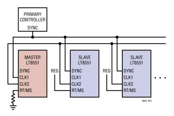
Figure 1. Clock Configuration in a Multiple LT8551 System
