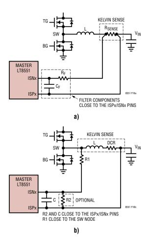
Figure 16. Inductor Current Sense Filter
