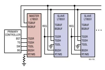
Figure 5. Gate Sensing in a Multiple LT8551 System
