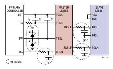
Figure 14. Gate Sensing Configuration with Filters and Schottky Clamps on TGSL
