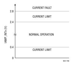
Figure 8. IAMP\_INTx Voltage for Current Limit and Current Fault
