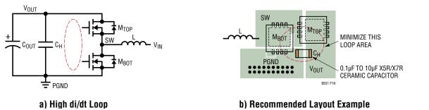
Figure 19. Minimize the High di/dt Loop Area in PCB Layout
