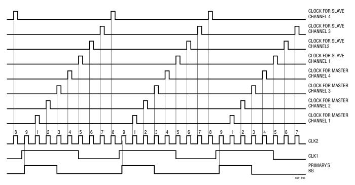
Figure 3. Clock Waveforms for a Two LT8551 System
