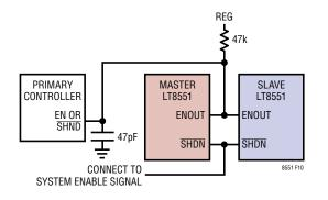
Figure 10. Recommended ENOUT Connection
