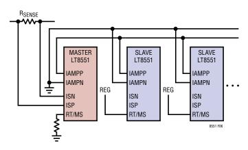
Figure 6. Primary Regulator's Switch Current Sensing in Multiple LT8551 System
