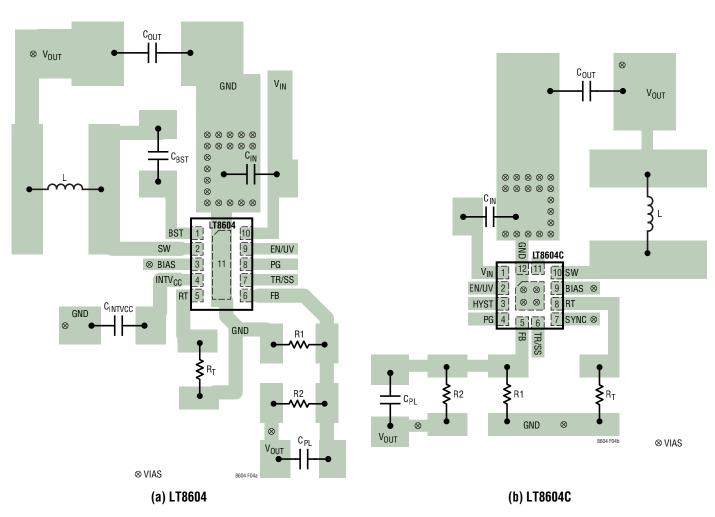
Figure 4. Recommended PCB Layout (Not to Scale)
