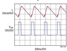
$24V_{IN}$  TO  $5V_{OUT}$  AT 0 mA  $R_T = 18.2k\Omega$ ,  $L = 47\mu$ H
