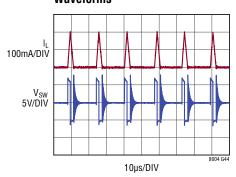
$12V_{IN}$  TO  $5V_{OUT}$  AT 20mA  $R_T = 18.2k\Omega$ ,  $L = 47\,\mu\text{H}$  SYNC = 0V
