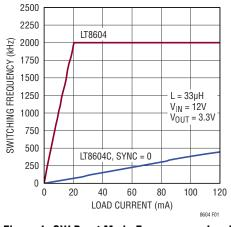
Figure 1. SW Burst Mode Frequency vs Load
