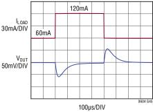
$12V_{IN}$  TO  $5V_{OUT}$ , LT8604C, SYNC FLOATING  $R_T=18.2\,k\Omega$ , L =  $47\mu H$ ,  $C_{OUT}=22\mu F$
