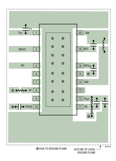
Figure 6. Recommended PCB Layout for the LT8630
