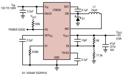
D1: VISHAY SS2PH10 L1: B65807JR49 EPCOS RM6 CORE WITH 0.2mm CENTERPOLE GAP NINE TURNS 60/38G LITZ WIRE
