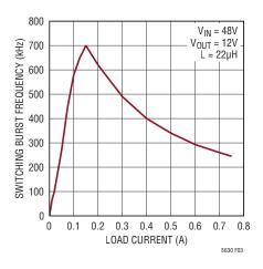
Figure 3. Frequency vs Load Current
