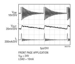
Figure 4. Burst Mode Operation
