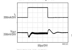
FRONT PAGE APPLICATION 200mA TO 600mA LOAD TRANSIENT  $\ensuremath{\text{V}_{\text{IN}}} = 48\ensuremath{\text{V}}$
