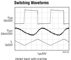
FRONT PAGE APPLICATION  $V_{IN} = 100V$  LOAD = 500mA
