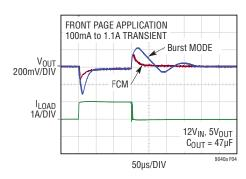
Figure 4. Load Step Transient Response with and without Forced Continuous Mode
