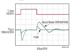
FRONT PAGE APPLICATION 100mA TO 1.1A TRANSIENT  $12V_{IN}$ ,  $5V_{OUT}$ ,  $f_{SW}$  = 1MHz  $C_{OUT}$  =  $100\mu F$
