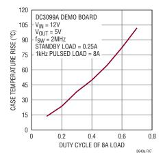
Figure 7. Case Temperature Rise vs 8A Pulsed Load
