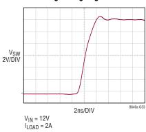
Switching Waveforms, Full Frequency Continuous Operation
