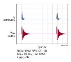
Figure 3. Burst Mode Operation
