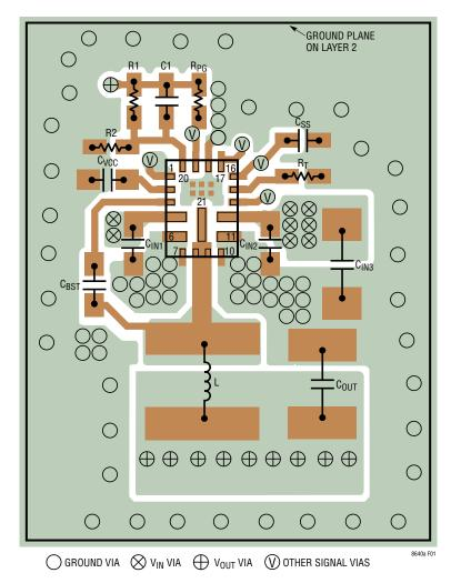
Figure 1. Recommended PCB Layout for the LT8640A
