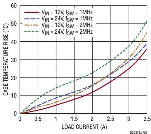
**Figure 2. DC2373A Temperature Rising vs Load Current**
