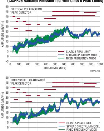
Figure 6. LT8644S Demo Circuit DC2779A EMI Performance
