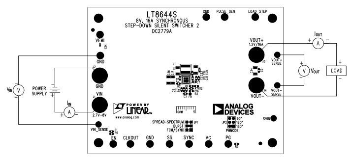
Figure 1. Proper Measurement Equipment Setup
