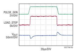
Figure 3. LT8644S Demo Circuit DC2779A Transient Response (V<sub>IN</sub> = 5V, 4A to 12A Load Step)
