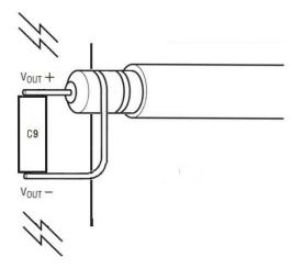
Figure 2. Measuring Output Ripple at Output Capacitor C9
