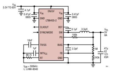
5V 8A Step-Down Converter with Soft-Start and Power Good
