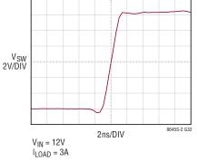
Switching Waveforms, Full **Frequency Continuous Operation**
