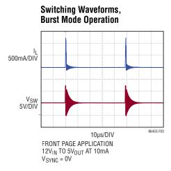
Figure 3. Burst Mode Operation
