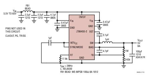
Ultralow EMI 5V, 8A Step-Down Converter with Spread Spectrum
