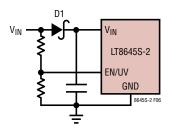
Figure 4. Reverse V<sub>IN</sub> Protection
