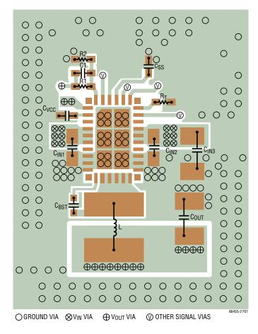
Figure 1. Recommended PCB Layout for the LT8645S-2
