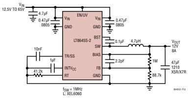
PINS NOT USED IN THIS CIRCUIT: CLKOUT, PG, SYNC/MODE
