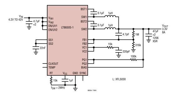
Two Phase, 3.3V, 8A, 2MHz Step-Down Converter
