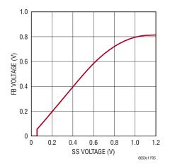
Figure 5. SS Pin Tracking
