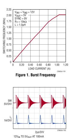
Figure 2. Burst Mode Operation
