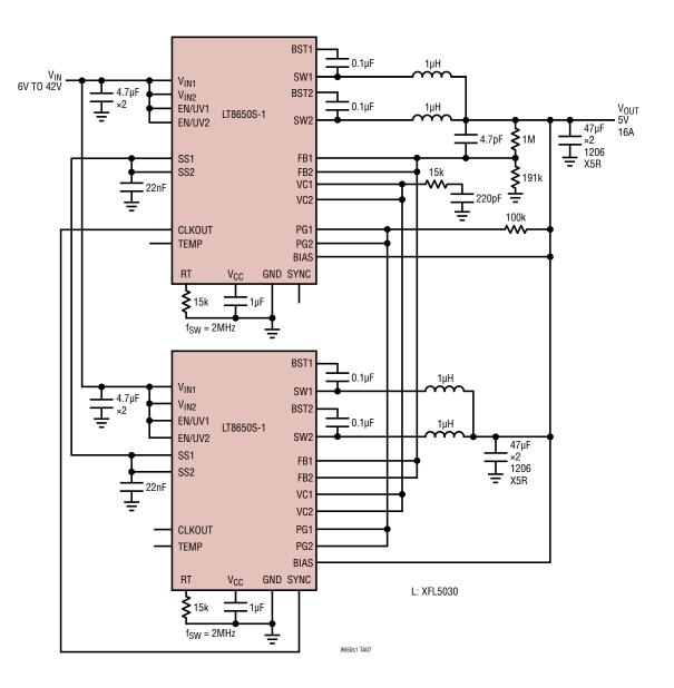
Four Phase, 5V, 16A, 2MHz Step-Down Converter
