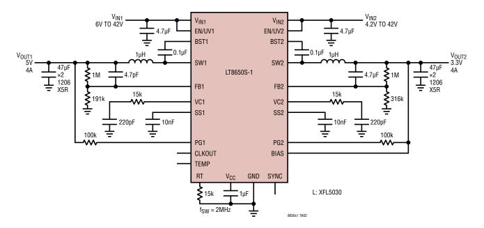
5V, 3.3V, 2MHz Step-Down Converter with FCM and External Compensation
