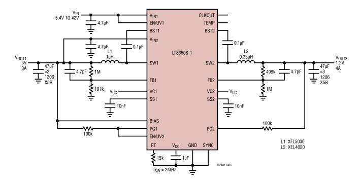
5V, 1.2V, 2MHz Two Stage Step-Down Converter with Output Sequencing
