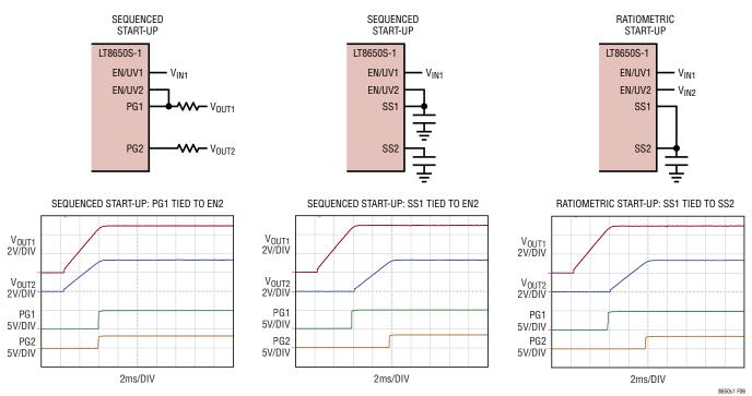
Figure 6. Sequencing and Start-Up Configurations
