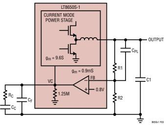
Figure 3. Model for Loop Response
