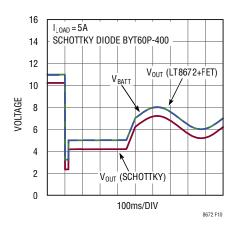
Figure 10. Automotive Cold Crank Waveforms
