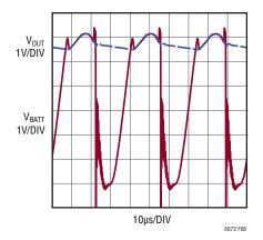
Figure 6. Rectification of Input Ripple Waveform (f = 30kHz, 5A Load Current)
