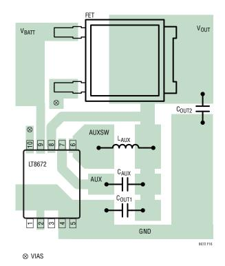
Figure 16. Recommended PCB Layout for the LT8672 (MSOP)
