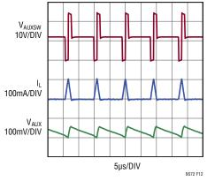
Figure 12. Auxiliary Boost Regulator Waveforms for 5mA Load on AUX
