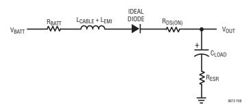
Figure 8. Simplified Application Model Including All Relevant Parasitics
