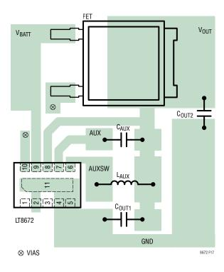
Figure 17. Recommended PCB Layout for the LT8672 (DFN)
