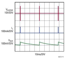
Figure 11. Auxiliary Boost Regulator Waveforms for 1µA Load on AUX (Steady State in Regulation)
