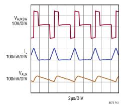
Figure 13. Auxiliary Boost Regulator Waveforms for 10mA Load on AUX
