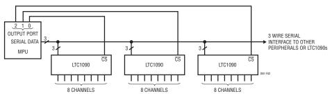
Figure 2. Several LTC1090s Sharing One 3 Wire Serial Interface
