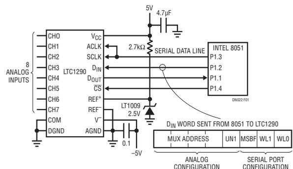
Figure 1. A Typical Hookup of the LTC1290
