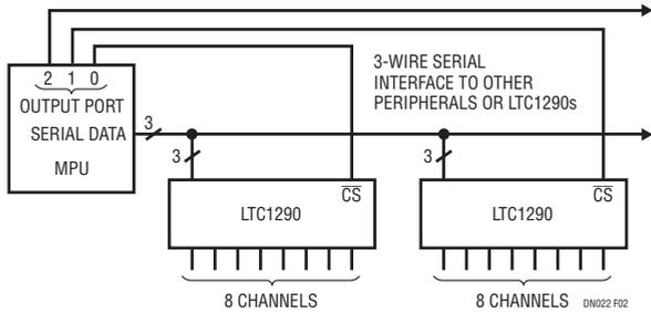
**Figure 2. Several LTC1290s Sharing One 3-Wire Serial Interface**
