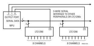
Figure 2. Several LTC1290s Sharing One 3-Wire Serial Interface
