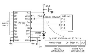
Figure 1. A Typical Hookup of the LTC1290
