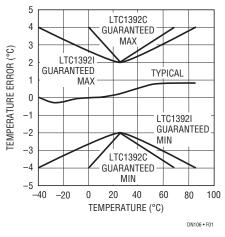
Figure 1. Output Temperature Error
