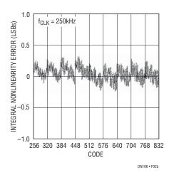
Figure 2b. Integral Nonlinearity, Power Supply Voltage Mode
