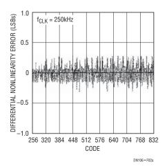
Figure 2a. Differential Nonlinearity, Power Supply Voltage Mode
