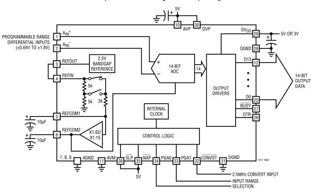
2.5Msps 14-Bit ADC with Programmable Input Range
