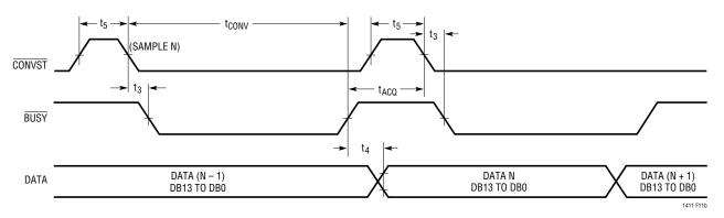
Figure 11b. CONVST Starts a Conversion with a Short Active High Pulse
