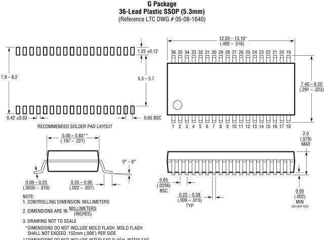
\*\*DIMENSIONS DO NOT INCLUDE INTERLEAD FLASH. INTERLEAD FLASH SHALL NOT EXCEED .254mm (.010") PER SIDE
