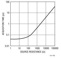
Figure 5. Acquisition Time vs Source Resistance
