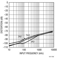
Figure 4. Distortion vs Input Frequency
