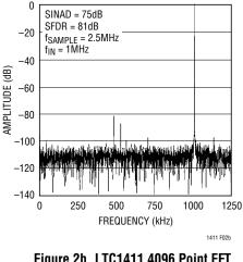
Figure 2b. LTC1411 4096 Point FFT, Input Frequency = 1MHz
