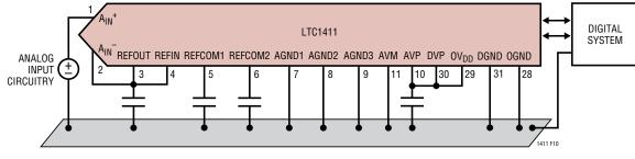
Figure 10. Power Supply Grounding Practice
