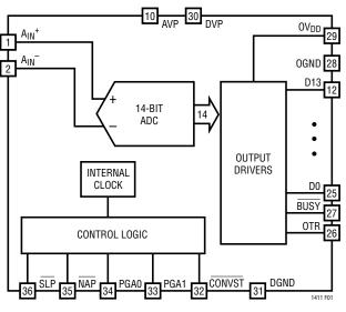
Figure 1. Simplified Block Diagram
