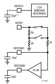
\*THIS PIN CAN BE TIED TO REFOUT OR AN EXTERNAL SOURCE \*\*A 22 $\mu\text{F}$  CAPACITOR IS NEEDED IF REFOUT IS USED TO DRIVE  $\text{Ain}^-$
