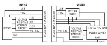
Figure 1. Block Diagram for the Device Bay
