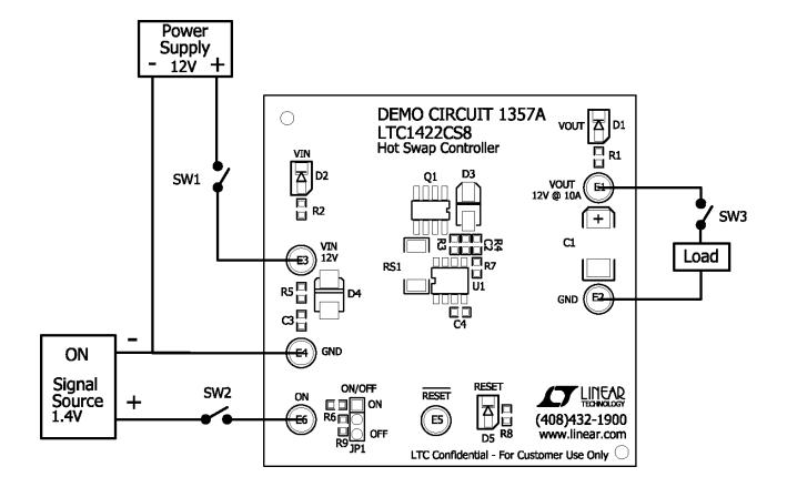
Figure 1. Proper Measurement Equipment Setup
