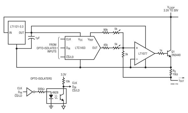
Figure 3. 4mA to 20mA Process Controller Has 3.3V Minimum Loop Voltage
