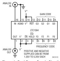
Figure 1. Dual Power Supply Circuit
