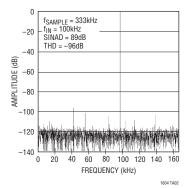
Figure 3. SINAD is Over 90dB and THD is –100dB at Low Input Frequencies. Even with 100kHz Inputs, SINAD Remains 89dB and THD is –96dB as Shown
