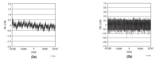
Figure 2. The LTC1604 Achieves Excellent INL (2a) and DNL (2b) without Cumbersome Autocalibration
