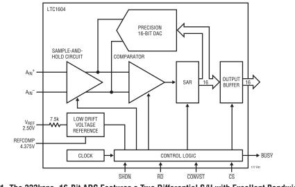
Figure 1. The 333ksps, 16-Bit ADC Features a True Differential S/H with Excellent Bandwidth and CMRR
