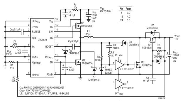
Figure 3. Synchronous 12V Output Buck/Boost Converter
