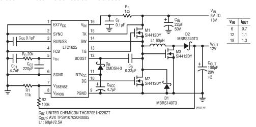
Figure 1. 12V Output Single Inductor Buck/Boost Converter
