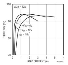
Figure 4. Efficiency of the Synchronous Buck/Boost Circuit
