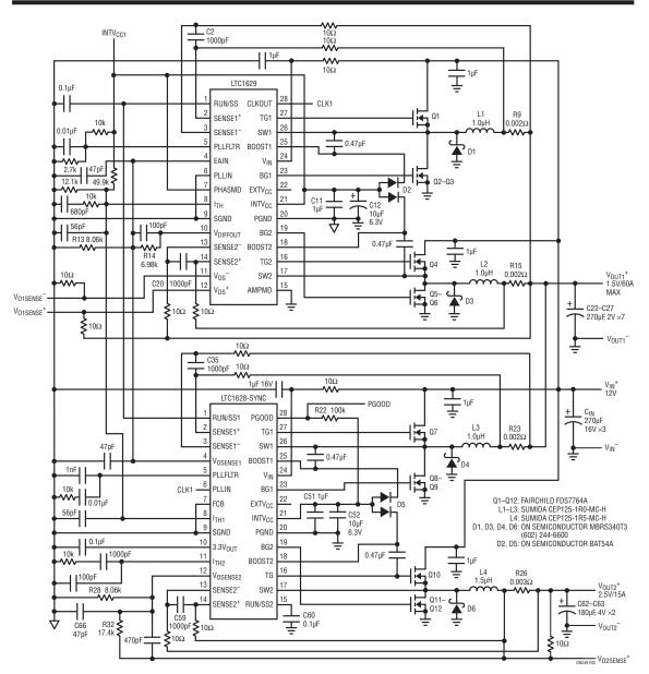
Figure 2. Schematic Diagram of 2-Output Circuit: Input 12V; Outputs 1.5V/60A, 2.5/15A
