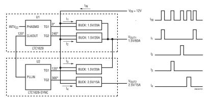
Figure 1. Block Diagram of 2-Output Power Supplies
