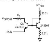
Figure 3. Optional Circuit to Modify Foldback Current Limit
