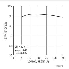
Figure 2. Efficiency vs Load Current
