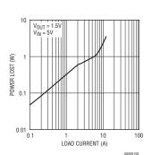
Figure 2. Power Loss Curve for 2-Step Regulator
