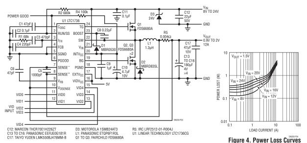
Figure 3. CPU Core Voltage Regulator for 1-Step Application
