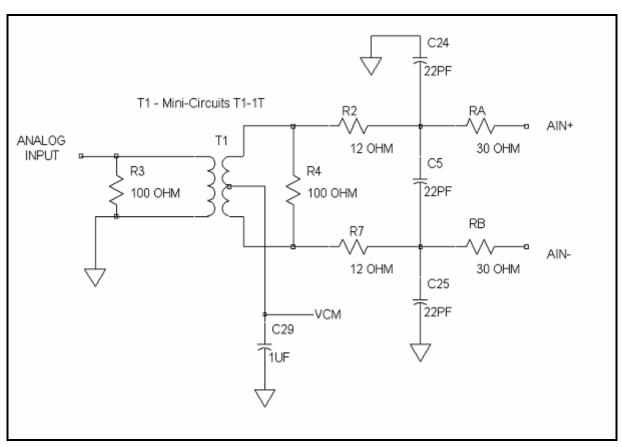
Figure 2. Analog Front End Circuit For A<sub>IN</sub> < 40MHz
