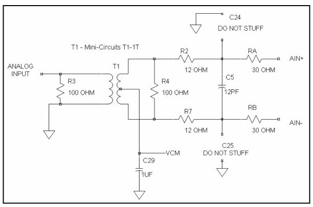
Figure 3. Analog Front End Circuit For 40MHz < AIN < 80MHz
