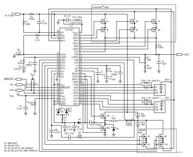
Figure 1. 4A Dual Battery System
