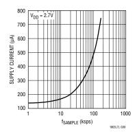
Figure 5. Supply Current vs f<sub>SAMPLE</sub>
