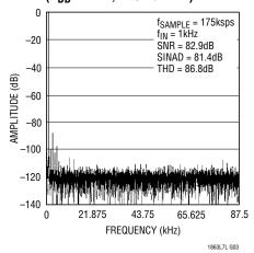
4096 Points FFT Plot (V<sub>DD</sub> = 3V, REFCOMP = Ext 3V)
