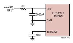
Figure 1a. Optional RC Input Filtering for Single-Ended Input
