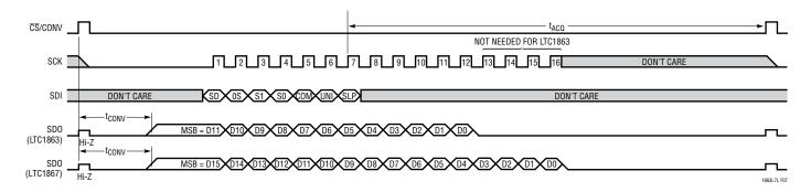
Figure 7. Example 2, CS/CONV Starts a Conversion With Short Active HIGH Pulse. With CS/CONV Returning LOW Before the Conversion, the ADC Remains Powered Up
