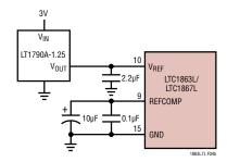
Figure 4b. Using the LT1790A-1.25 as an External Reference
