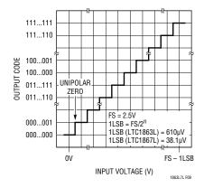
Figure 9. LTC1863L/LTC1867L Unipolar Transfer Characteristics (Straight Binary)
