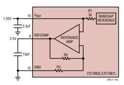
Figure 4a. LTC1867L Reference Circuit
