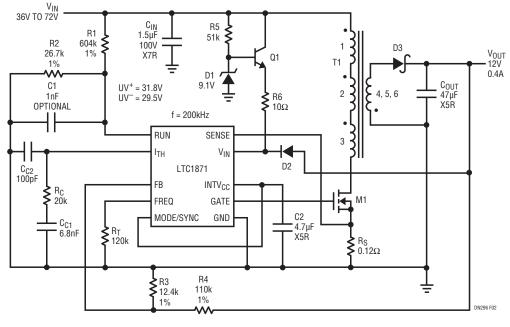
T1: COILTRONICS VP1-0076 (3 WINDINGS IN SERIES ON PRIMARY, 3 IN PARALLEL ON SECONDARY)
