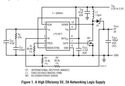
were chosen for the 2A output current level, and a low ESR ceramic output capacitor keeps the output ripple below  $60mV_{P-P}$ .
