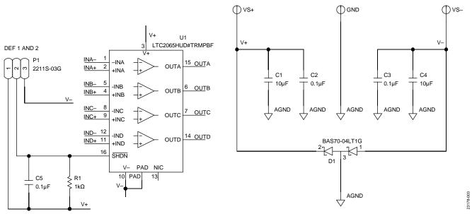
Figure 3. EVAL-LTC2065/LTC2068-TQFN Schematic, Page 1
