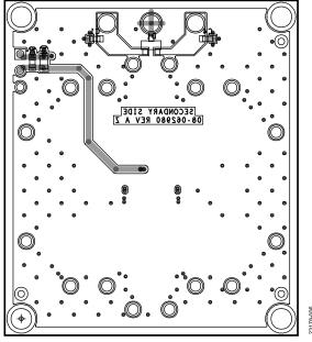
Figure 6. EVAL-LTC2065/LTC2068-TQFN Layout Pattern, Secondary Side
