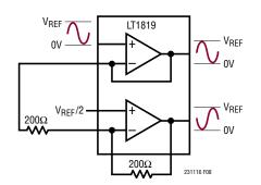
Figure 8. Single-Ended to Differential Driver
