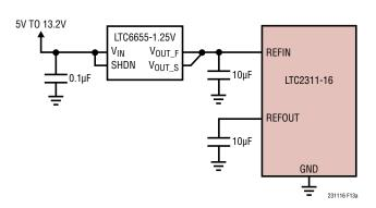
Figure 13a. LTC2311-16 with an External REFIN Voltage
