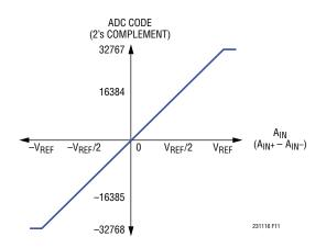
Figure 11. Fully-Differential Transfer Function
