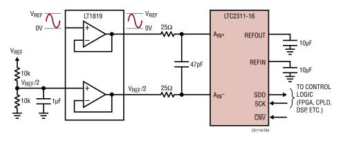
Figure 4. Pseudo-Differential Bipolar Application Circuit
