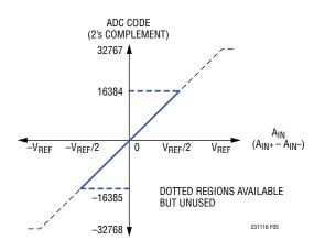
Figure 5. Pseudo-Differential Bipolar Transfer Function
