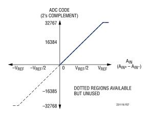
Figure 7. Pseudo-Differential Unipolar Transfer Function
