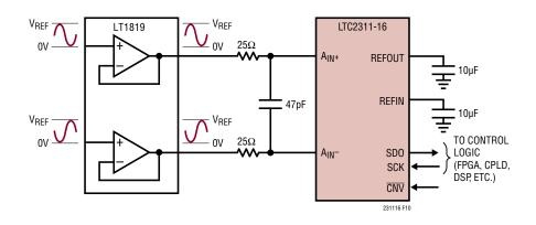
Figure 10. Fully-Differential Application Circuit
