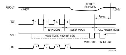
Figure 19. CMOS Mode SLEEP and WAKE Using SCK
