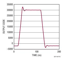
Figure 15. Transient Response of the LTC2311-16
