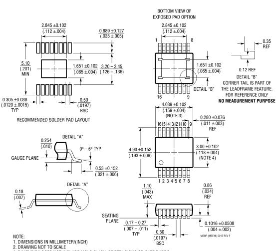
**MSE Package** 16-Lead Plastic MSOP, Exposed Die Pad (Reference LTC DWG # 05-08-1667 Rev F)
