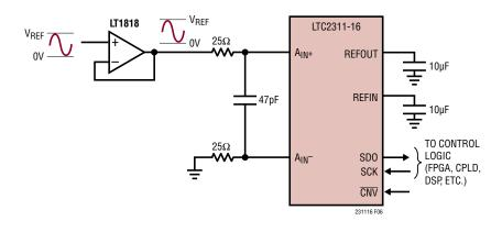
Figure 6. Pseudo-Differential Unipolar Application Circuit
