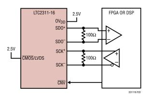
Figure 22. LTC2311-16 Using the LVDS Interface
