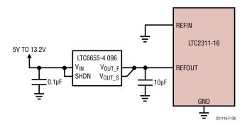
Figure 13b. LTC2311-16 with an External REFOUT Voltage
