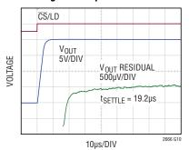
±10V RANGE; INTERNAL REFERENCE RISING 20V STEP; AVERAGE OF 64 EVENTS FALLING SETTLING IS SIMILAR OR BETTER RESIDUAL WAVEFORM INCLUDES 100ns FIXTURE DELAY
