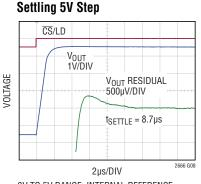
OV TO 5V RANGE; INTERNAL REFERENCE RISING 5V STEP; AVERAGE OF 128 EVENTS FALLING SETTLING IS SIMILAR OR BETTER RESIDUAL WAVEFORM INCLUDES 100ns FIXTURE DELAY
