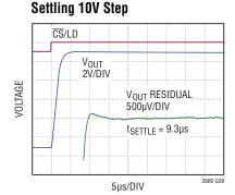
OV TO 10V RANGE; INTERNAL REFERENCE RISING 10V STEP; AVERAGE OF 128 EVENTS FALLING SETTLING IS SIMILAR OR BETTER RESIDUAL WAVEFORM INCLUDES 100ns FIXTURE DELAY
