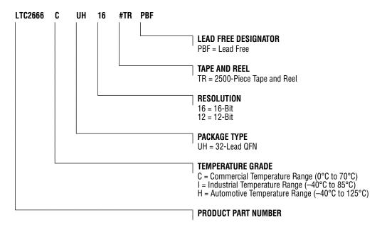
Contact the factory for parts specified with wider operating temperature ranges. \*The temperature grade is identified by a label on the shipping container.
