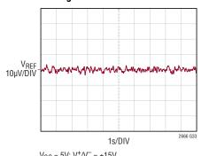
$V_{CC} = 5V$ ;  $V^+/V^- = \pm 15V$  $V_{REF} = 2.5V$  (INTERNAL REFERENCE)  $C_{REF} = C_{REFCOMP} = 0.1 \mu F$
