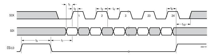
Figure 1. Serial Interface Timing
