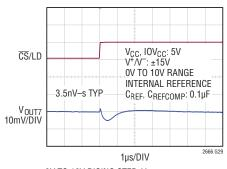
OV TO 10V RISING STEP: V<sub>OUTO</sub> MEASURED CHANNEL: V<sub>OUT7</sub>
