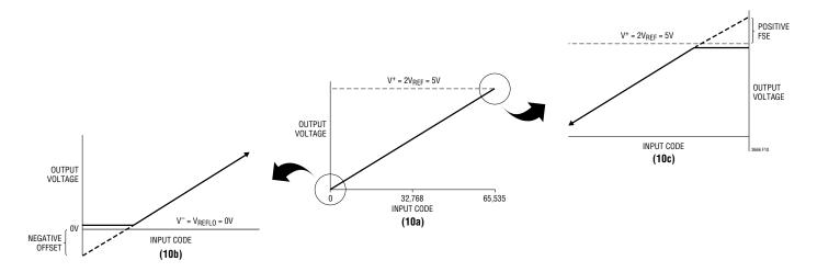
Figure 10. Effects of OV to 5V Output Range for Single-Supply Operation. (10a) Overall Transfer Function (10b) Effect of Negative Offset for Codes Near Zero-Scale (10c) Effect of Positive Full-Scale Error for Codes Near Full-Scale
