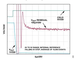
Figure 32. Settling Time, 5 V (Falling)
