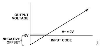
Figure 53. Effects of 0 V to 5 V Output Range for Single-Supply Operation, Overall Transfer Function
