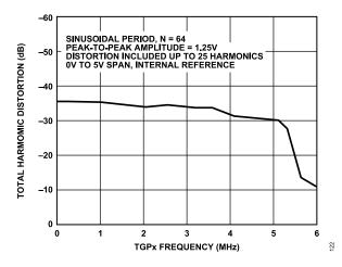
Figure 22. Total Harmonic Distortion vs. TGPx Frequency
