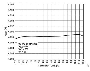
Figure 7. V<sub>REF</sub> vs. Temperature
