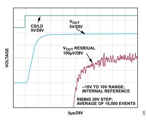
Figure 35. Settling Time, 20 V
