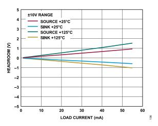
Figure 40. Vx<sup>+</sup>/V<sup>-</sup> Bipolar Headroom vs. Output Load Current
