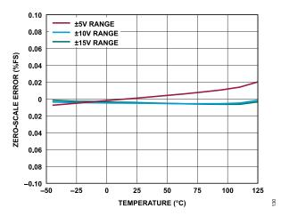
Figure 30. Zero-Scale Error vs. Temperature
