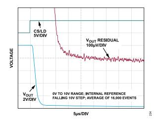
Figure 34. Settling Time, 10 V (Falling)
