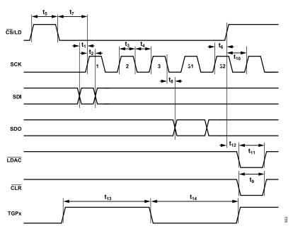
Figure 2. Serial Interface Timing Diagram
