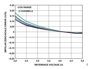
Figure 5. Bipolar Zero-Scale Error vs. V<sub>REF</sub>
