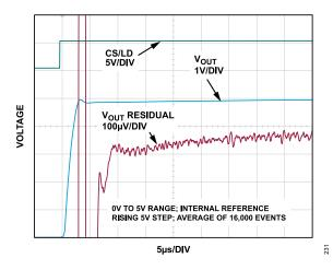
Figure 31. Settling Time, 5 V
