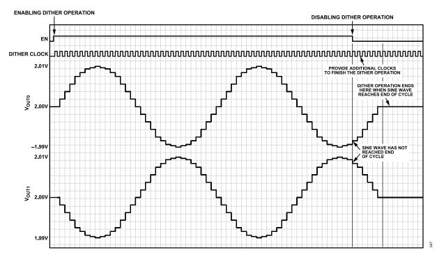
Figure 52. Termination of Sinusoidal Dither Waveforms
