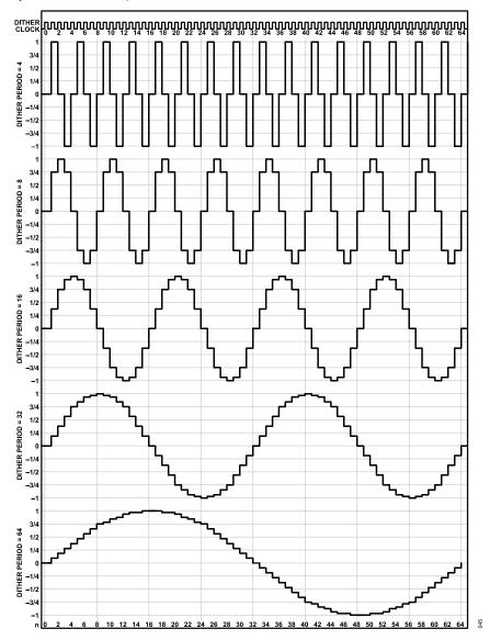
Figure 50. Sinusoidal Waveforms for Various Values of Dither Period N
