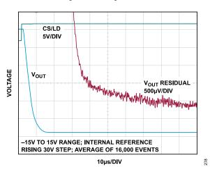
Figure 38. Settling Time, 30 V (Falling)
