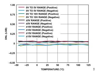
Figure 28. DNL vs. Temperature
