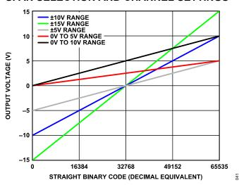
Figure 46. DAC Transfer Functions, All Voltage Spans and Bit Resolutions, Internal Reference Mode
