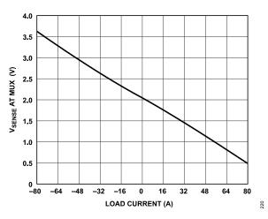
Figure 20. V<sub>SENSE</sub> at MUX vs. Load Current
