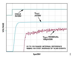
Figure 33. Settling Time, 10 V
