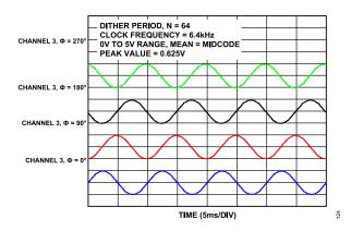
Figure 24. Sinusoidal Dither for Various Phase Settings
