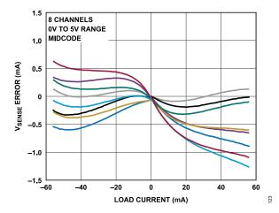
Figure 23. V<sub>SENSE</sub> Error vs. Load Current from Equation 2 and Equation 3
