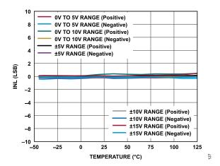
Figure 27. INL vs. Temperature
