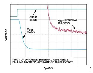
Figure 36. Settling Time, 20 V (Falling)
