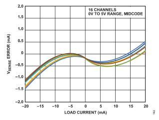
Figure 41. V<sub>SENSE</sub> Error vs. Load Current from Equation 5
