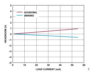
Figure 39. Vx<sup>+</sup>/V<sup>-</sup> Unipolar Headroom vs. Output Load Current
