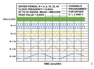
Figure 19. Sinusoidal Dither Waveform
