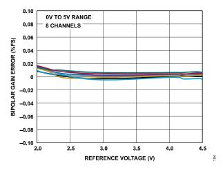
Figure 4. Bipolar Gain Error vs. V<sub>REF</sub>
