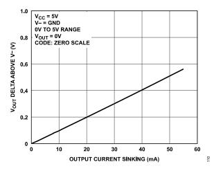
Figure 10. V<sub>OUT</sub> Delta Above V<sup>-</sup> vs. Output Current Sinking
