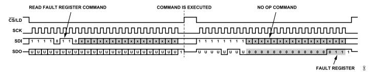
Figure 45. Typical Read Command Sequence for 24-Bit Words
