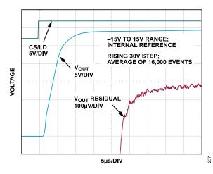
Figure 37. Settling Time, 30 V
