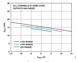
Figure 12. I<sub>VCC</sub> vs. V<sub>OUT</sub>
