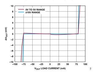
Figure 18.  $\Delta V_{OUT}$  vs.  $V_{OUT}$  Load Current
