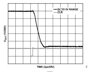
Figure 13. Hardware CLR to Zero Scale
