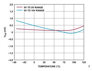
Figure 8. Unipolar Offset Error (Vos) vs. Temperature
