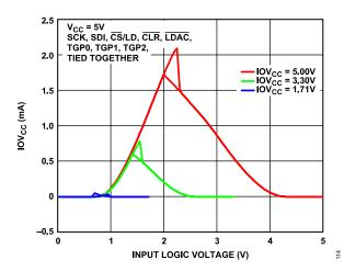
Figure 14. IOV<sub>CC</sub> vs. Input Logic Voltage
