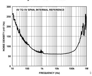
Figure 17. Noise Density vs. Frequency
