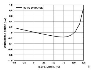
Figure 6. Zero-Scale Error (ZSE) vs. Temperature
