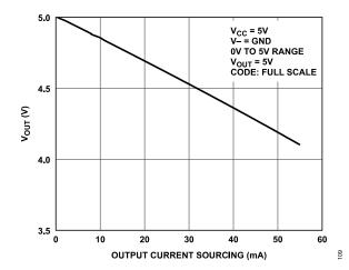
Figure 9. V<sub>OUT</sub> vs. Output Current Sourcing
