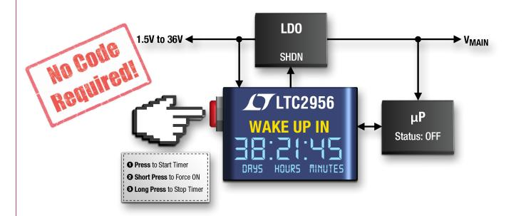
The LTC<sup>®</sup>2956 Wake-Up Timer provides a periodic on/off signal, waking up a system to perform routine tasks (such as measuring a sensor or capturing images) while keeping it off most of the time to save power. While "sleeping," the LTC2956 sips only 800nA of quiescent current from a battery or rail.
