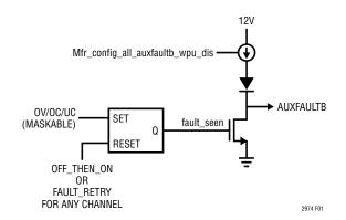
Figure 1. AUXFAULTB MUX
