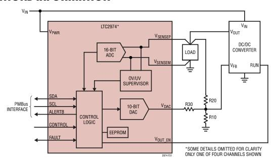
Figure 31. Application Circuit for DC/DC Converters with External Feedback Resistors
