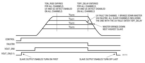
Figure 19. Fault on Channel 1 Tracking All Supplies Down
