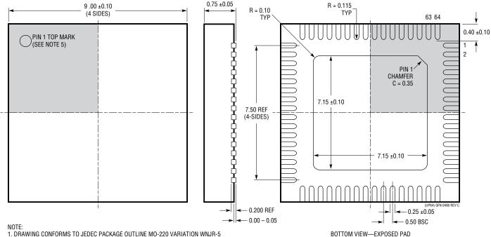
1. DRAWING CONFORMS TO JEDEC PACKAGE OUTLINE MO-220 VARIATION WNJR-5 2. ALL DIMENSIONS ARE IN MILLIMETERS 3. DIMENSIONS OF EXPOSED PAD ON BOTTOM OF PACKAGE DO NOT INCLUDE
