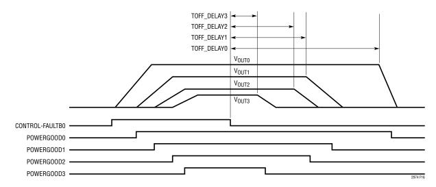
Figure 16. Cascade Sequence ON with Time Based Sequence Down on FAULTO
