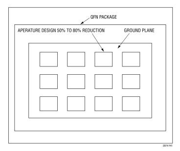
Figure 41. Suggested Screen Pattern for Die Attach Pad
