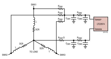
Figure 35. Multiphase DCR Current Sensing Circuits
