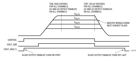
Figure 18. Control Pin Tracking All Supplies Up And Down
