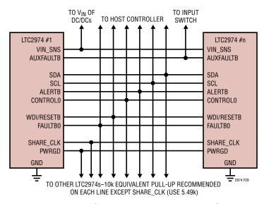
Figure 29. Typical Connections between Multiple LTC2974s
