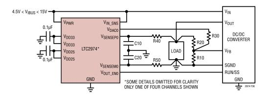
Figure 36. Anti-Aliasing Filter on V<sub>SENSE</sub> Lines
