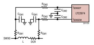
Figure 34. DCR Current Sensing Circuits
