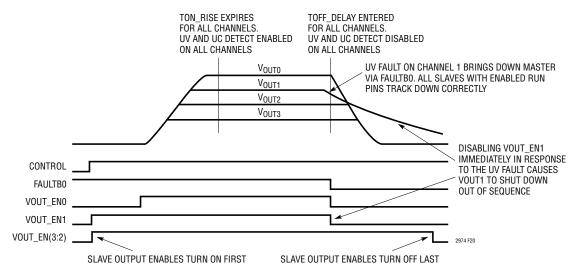
Figure 20. Improperly Configured Fault Response on Faulting Channel Disrupts Tracking
