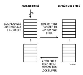
Figure 22. Fault Logging
