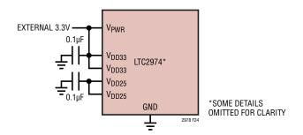
Figure 24. Powering LTC2974 from External 3.3V Supply
