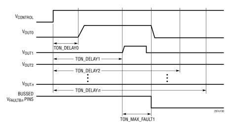
Figure 30. Aborted On-Sequence Due to Channel 1 Short
