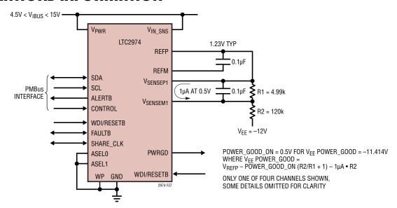
Figure 37. Sensing Negative Voltages
