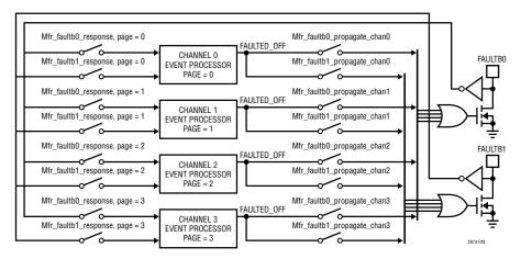
Figure 28. Channel Fault Management Block Diagram
