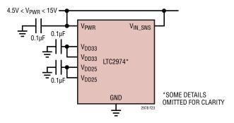
Figure 23. Powering LTC2974 Directly from an Intermediate Bus
