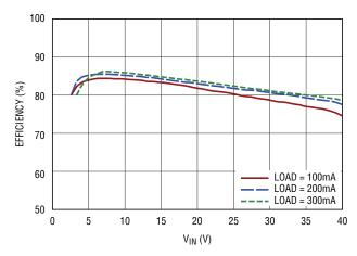
Figure 2. DC1687B Efficiency in Burst Mode Operation
