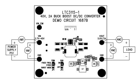
Figure 3. Proper Measurement Equipment Setup
