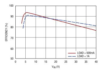
Figure 1. DC1687B Efficiency in PWM Mode
