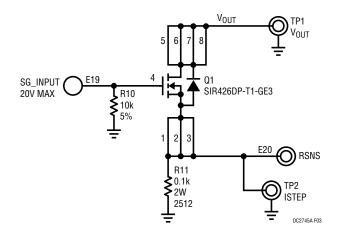
Figure 3. Optional Transient Response Circuit
