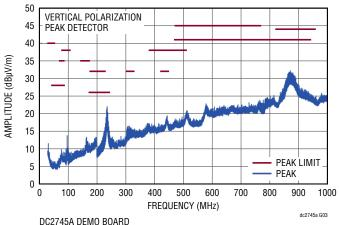
DC2745A DEMO BOARD (WITH EMI FILTER INSTALLED) 3.3V INPUT TO 1.2V OUTPUT AT 4.8A, f<sub>SW</sub> = 2MHz
