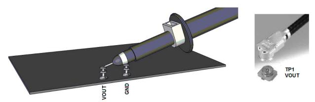
Figure 2. Technique for Measuring Output Ripple and Step Response a) With a Scope Probe.
