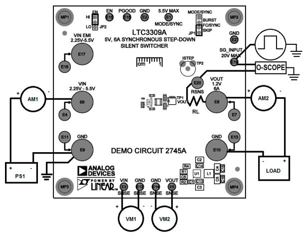
Figure 1. Test Setup for the DC2745A Demo Board
