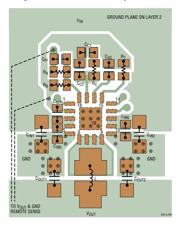
Figure 4. Recommended PCB Layout for the LTC3311
