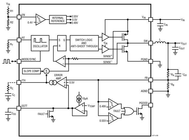
$^{\star}$ ON THE LTC3311-X, THE R $_{\!A}$  and R $_{\!B}$  resistors are internal, along with C $_{\!F\!F}$
