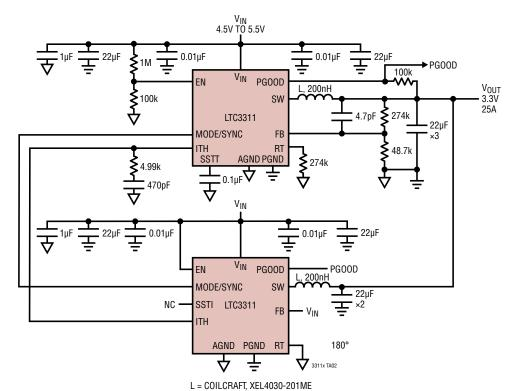
Three Phase, 2MHz, 0.6V, 37.5A, Forced Continuous Mode
