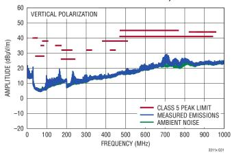
DC3056A DEMO BOARD (WITH EMI FILTER INSTALLED) 3.3V INPUT TO 1.2V OUTPUT AT 10A, f<sub>SW</sub> = 2MHz
