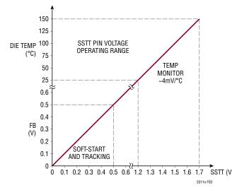
Figure 3. Soft-Start and Temperature Monitor Operation
