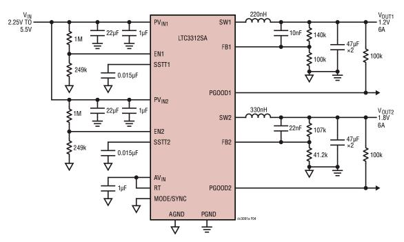
Figure 4. LTC3312SA Dual 6A Buck Typical Application Schematic
