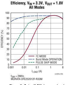
Figure 6. Output2 Efficiency vs Load
