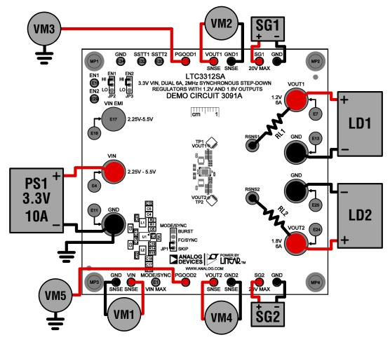
Figure 2. Test Setup for DC3091A Demo Board
