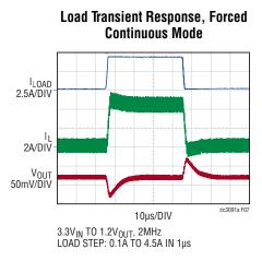
Figure 7. Output1 Load Step Response
