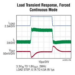
Figure 8. Output2 Load Step Response
