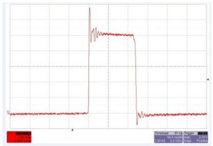
Figure 2: Buck regulator switching @2MHz with full speed rise & fall times Click on image to enlarge
