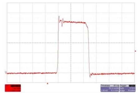
Figure 3: Buck regulator switching @2MHz, reduced speed rise & fall times Click on image to enlarge
