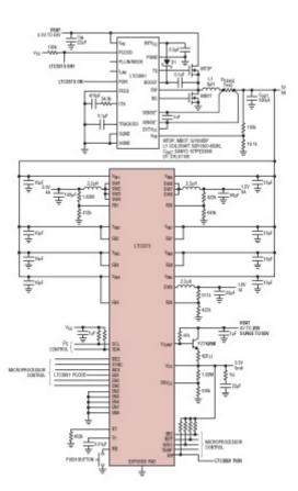
Figure 6: LTC3375 driven by a high voltage upstream buck converter Click on image to enlarge
