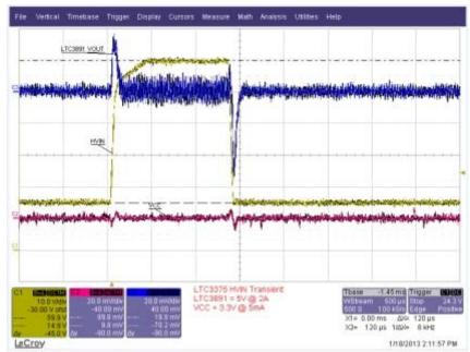
Figure 5: LTC3375 high voltage transient performance Click on image to enlarge
