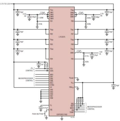
Figure 1: LTC3375 simplified 3-output 4A / 3A / 1A block diagram Click on image to enlarge
