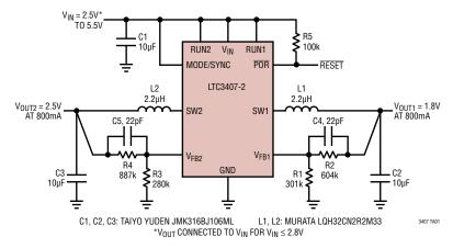
Figure 1. 2.5V/1.8V at 800mA Step-Down Regulators
