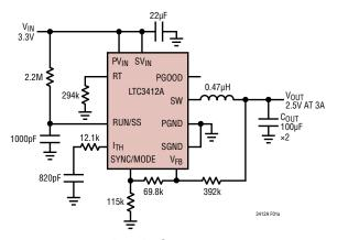
Figure 1. 2.5V/3A Step-Down Regulator
