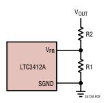
Figure 2. Setting the Output Voltage
