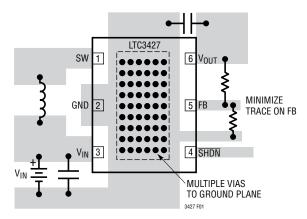
Figure 1. Recommended Component Placement for a Single Layer Board. Traces Carrying High Current are Direct (GND, SW,  $V_{IN}$ ,  $V_{OUT}$ ). Trace Area at FB is Kept Low. Lead Length to Battery Should be Kept Short.  $V_{IN}$  and  $V_{OUT}$  Ceramic Capacitors Should be as Close to the LTC3427 as Possible. A Multilayer Board with a Separate Ground Plane is Ideal, but not Absolutely Necessary
