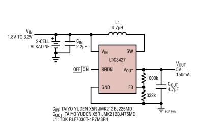
Figure 4. 2-Cell Alkaline to 5V Synchronous Boost Converter with Output Disconnect
