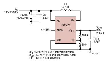
Figure 3. 2-Cell Alkaline to 3.3V Synchronous Boost Converter
