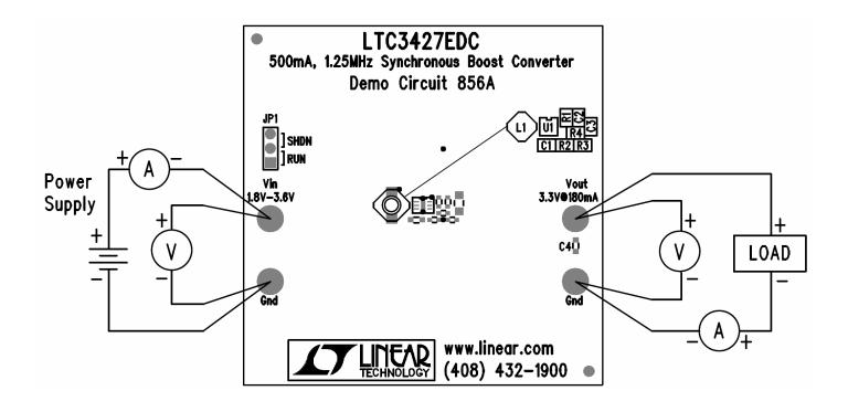
Figure 1. Proper Measurement Equipment Setup
