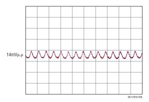
Figure 5. Output Noise,  $V_{IN} = 4.5V$ ,  $I_{OUT} = 1A$
