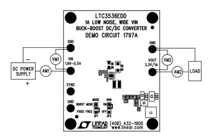
Figure 1. Proper Measurement Equipment Setup
